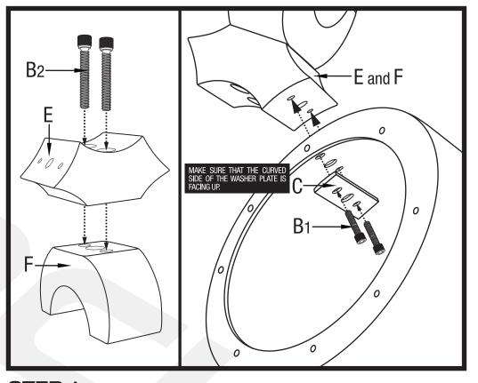
**STEP 1** Remove the top half of the clamp. Attach the bottom half of the clamp to the speaker interconnect using B2 bolts. Use the B1 bolts and the washer plates to attach one speaker can to each side of the speaker bridge. Make sure that the curved side of the washer plate is facing up.
