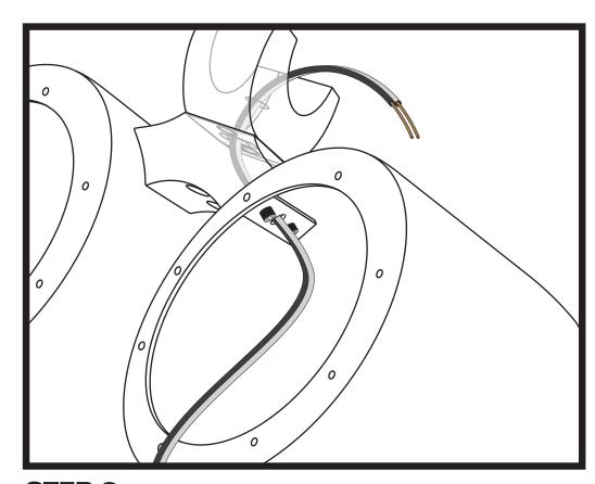
**STEP 2** Thread the speaker wire through the predrilled center hole and out through the clamp as shown in the illustration. Repeat for the second can.
