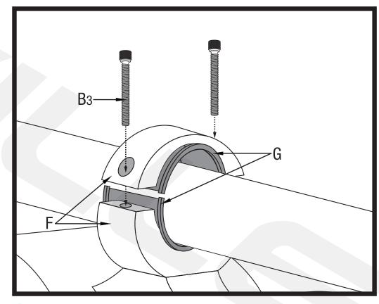
**STEP 4** If your wake tower has predrilled holes for routing speaker cables, insert the cables at this time. If the clamp does not fit snugly, use one of the 4 included rubber inserts. Place the top half of the clamp over the wake tower pole and attach to the lower half. Do not overtighten the screws. If you need an insert other than the ones that are included, email us at: sales@rockvilleaudio.com.
