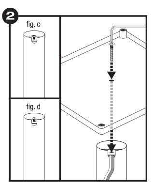
Remove the socket head screws from the ends of the stand body (figs. c and d). Turn the base plate upside down and align the hole in the center of the base plate with one of the holes on either end of the stand body. Insert a screw and use the Allen key to tighten it. Do not overtighten.
