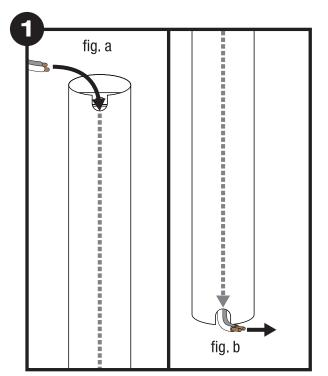
First, feed the speaker cable into the u-shaped opening on the top of the stand body (fig. a) and bring it back out through the u-shaped opening at the bottom (fig. b).
