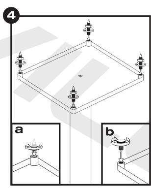
To place the stand on a carpeted floor, use the brass isolation spikes. Screw the spikes to the corresponding openings at each corner of the bottom of the base plate. Adjust the height as needed to keep the stand level. Use the nut to secure the spike's position (inset a). For wood, laminate, tile, or bare floor, use the included rubber feet (inset b).
