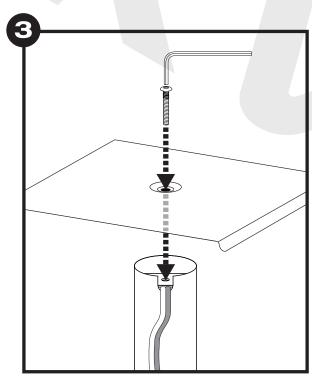
Turn the partially assembled stand over and set it down. With the indentation facing down, align the plate so that the indentation sits in the opening of the stand body. Insert the other screw and use the Allen key to tighten it. Do not overtighten.
