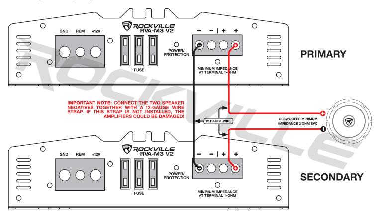
The RVA-M3 V2 is shown for display purposes. All configurations and wiring instructions also apply to the RVA-M2.
