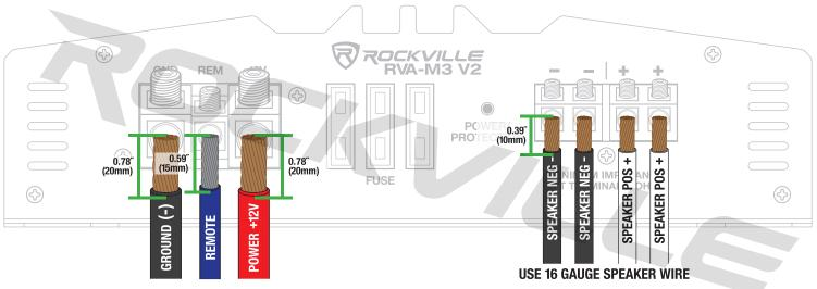
**TERMINAL DIAMETER:** POWER =  $\Phi$ 0.33in (8.5mm), REM =  $\Phi$ 0.15in (4mm), SPEAKER =  $\Phi$ 0.15in (4mm) **TERMINAL DEPTH:** POWER = 0.78in (20mm), REM = 0.59in (15mm), SPEAKER = 0.39in (10mm)
