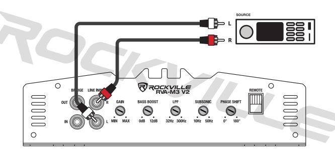
These amps are 1 ohm stable monoblock amplifiers. No matter how many woofers you choose to wire up to these models, the final impedance should not fall below 1 ohm. Please see pages 15 and 16 for various speaker impedance configurations.
